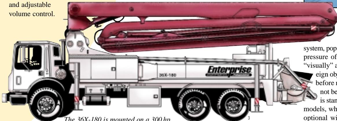
The 36X-180 is mounted on a 300 hp Mack MR 690S chassis with fully hydraulic outriggers.
