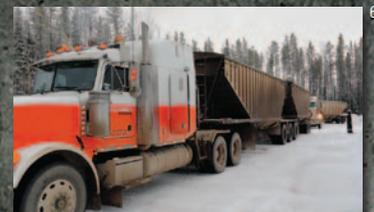
Pneumatic bulk handling trailers have been replaced with more readily available double drop grain trailers that are less costly to operate. This allows greater flexibility in scheduling as well as lowered demurrage costs associated with the loading and unloading cycle.
