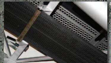
A Chevron belt pattern effectively conveys fracking sand.
