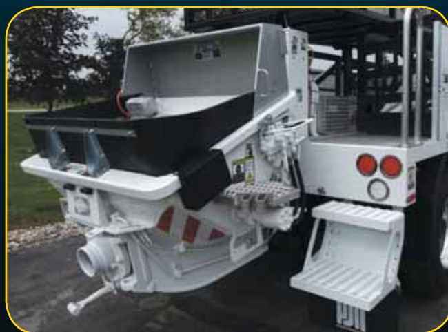
Large capacity hopper and breakaway rear steps
