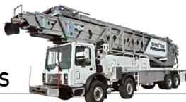
Only Putzmeister gives operators the choice to place concrete with a telescopic belt conveyor. Putzmeister's line of Telebelts® ranging from the TB 110 to the TB 200 with truck, semi-trailer, tower and crane chassis mounting configurations, gives operators the flexibility to easily switch from placing concrete to rock, stone, gravel or backfill. They handle concrete mixes with any size slump and materials ranging from sand to 6-inch aggregate.
