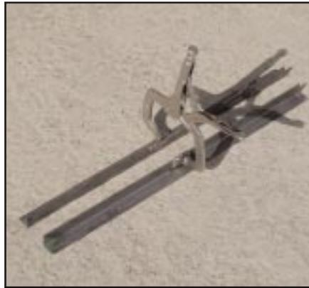
The above is an example of a velocity brake that you can create. Utilize a simple pair of welding vise grips that have the small swivel pads on the clamp jaws. Take two pieces of 1" x 1" angle iron, each two feet long. Weld the angle iron to the pads as shown in the photo.
