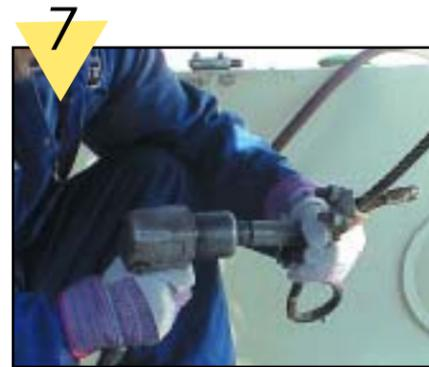
Remove the cable clamps and thimble from the end of the cable. If the cable has a swaged socket, cut the socket off. Be sure to melt the cable strands together at the cut to prevent the cable from unraveling (see above).
