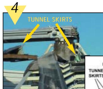
Remove the tunnel skirts and move the belt to one side, tying it out of the way.
