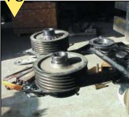
Shown is the top plate removed. The bearings are still inside (under) the top mount. The sheaves can now be removed, one at a time. Small pry bars will usually accomplish this quite effectively.
