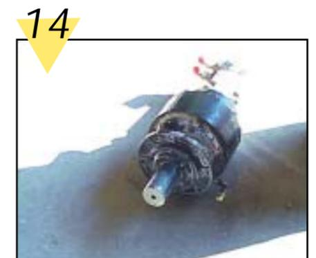
Mark the gear reducer housing and drive plate for alignment. Remove the bolts (item #19) from the gear reducer and separate the gear reducer and motor from the drive sheave plates. It is not necessary to separate the motor from the reducer.
