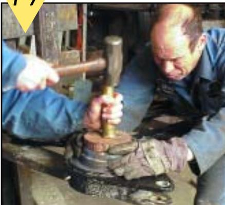
Reassemble by following the above steps in reverse. Replace bearings as needed. They are not a tight fit but must go in straight. After the unit is reassembled and the plate spacers (item #10 in Illustration B) are bolted in, check that the sheaves can be turned by hand. Make sure bolts (items #15 and #18) are also not overtightened. If the above steps have been followed and they still do not turn easily by hand, one spacer
