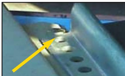
**Note: You must place a bolt in the first hole of the track. This is to keep the take-up from falling out of the slot at the rear of the track (see arrow).**
