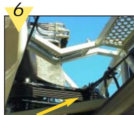
Remove the clevis that attaches the cable to the deadhead of the telescope drive assembly (TB 105) or the space tensioner (TB 130). If the cable has a swaged socket end, remove the socket pin.
