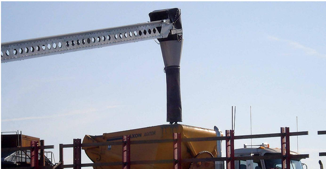
“The Telebelts convey and place the concrete into either loading trucks, or into hoppers of our large-scale conveyors,” comments Schermerhorn.
