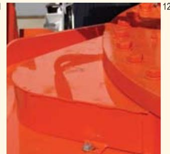
Putzmeister is constantly working on ways to ease maintenance and enhance performance of its Telebelt models. This includes a new three-piece cover for the slewing gear on the TB 110.
