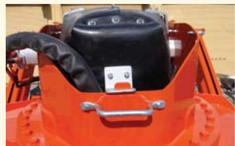
When properly installed, the bracket on the feeder boot should look like this.
