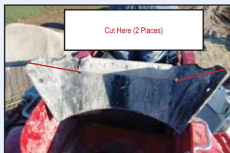
Cuts in the feeder scraper skirt should start at the skirt notch at the ends of the skirt clamp.
