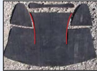
The side slits on the TB 110 transfer splatter flap need to be longer.
