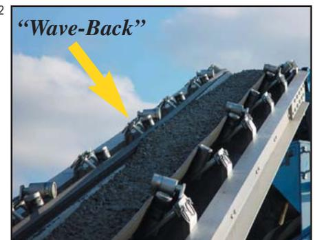
To reduce "wave-back", achieve greater belt utilization and keep the belt cleaner, the belt speed and ready-mix discharge flow must be altered. Various alternatives include increasing belt speed, reducing mixer output or doing both.
