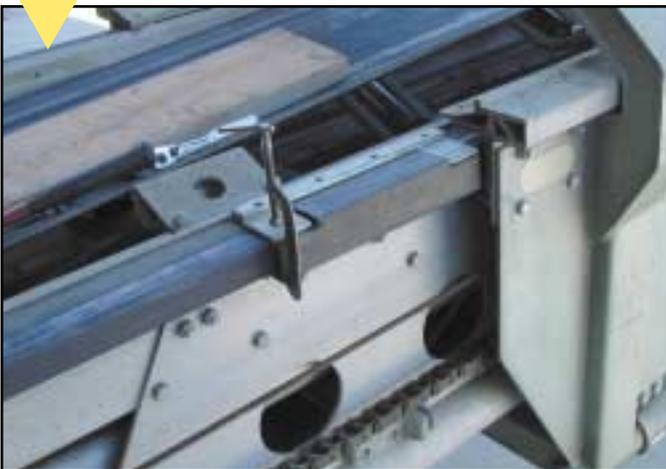
Telescope the boom out and let the clamp pull the guide block and retainer out.
