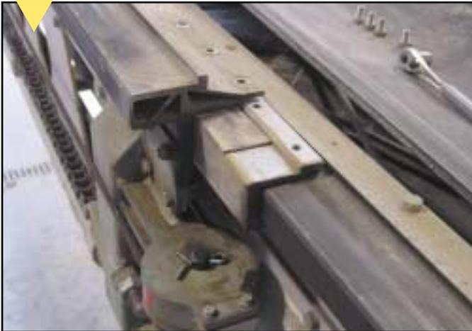
Only replace one guide block at a time. Remove the four bolts from the retainer. Apply enough down pressure on the saw horse to slightly lift the boom section in the guide block. When the guide block is loose, you can reach behind the retainer and knock the retainer and guide block out with a punch.
