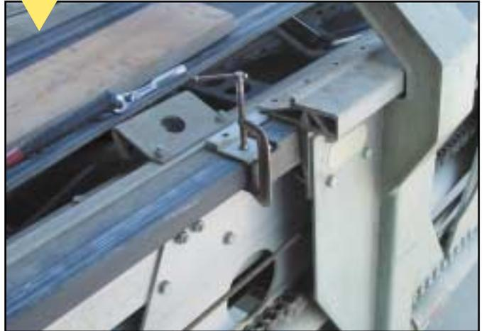
Sometimes, this little trick will work ... when the retainer and guide block have been pushed out a little ways, clamp them with a C-clamp. You can then proceed to step five.
