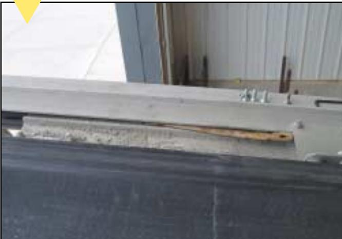
A flat wall tie makes a suitable punch for working with the male guide blocks. Use down pressure to center the rail when inserting the new slides. Use a C-clamp to pull the rails sideways, if needed. DO NOT overtighten the retainer bolts. They will firm up when the head is recessed about 1/8" into the plastic. This is sufficient.
