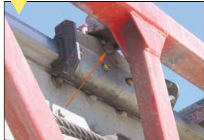
Replacement of TB-105 and TB-130 **rocker arm guide blocks** is fairly straightforward. Fully retract the boom so the aluminum sections are resting on the bottom slides. Remove the cotter key and pin (arrow) and slide the assembly out of position. Replace the guide block and reinstall the assembly.
