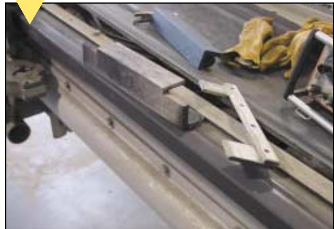
Remove the retainer and guide block.
