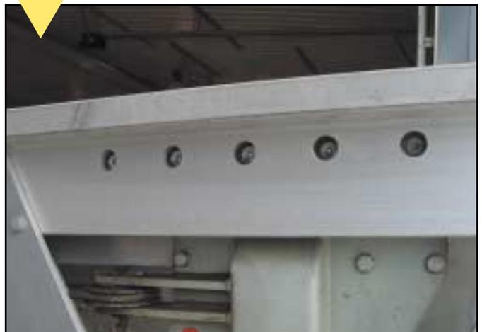
TB-105 male guide blocks have four mounting holes while the TB-80 and TB-130 have five. There are only three access holes on the TB-80 B arm, so you have to remove three bolts, then telescope the boom to get to the other two. All other access points have the equal corresponding number of holes.
