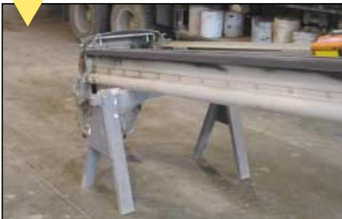
First, find something strong to rest the end of the boom on or you could damage it. A strong saw horse or a 55 gallon drum and some wooden blocks usually are sufficient. Position the “rest” so the scraper and bottom rollers are not on it. Throughout this replacement process, lubricate the female channels wherever the guide blocks contact the aluminum.
