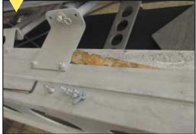
To remove the male guide blocks, remove the retainer bolts. Apply down pressure on the tip of the boom until the guide block is loose. Tap the guide block out with a punch. The retainer can remain in the rail, just don't let it slide out of reach. If you want to make sure it doesn't get away from you, use a piece of wire with a hook bent at the end to hold the retainer in place.
