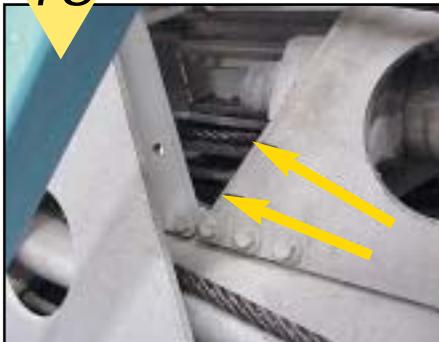
Remove the guide clevis and bar which were inserted in previous steps. Cut the cables apart at the weld joint.
