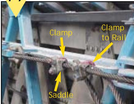
Pass the end of the cable around the take-up sheave. Form a loop with a cable clamp and pull the cable snug with the tension cylinder. Make sure the clamps are installed with the saddle on the "live" end of the cable.
