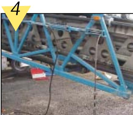
4 Completely release cable tension and disconnect the cable, as shown. Remove the cable clamps and pull the cable out of the 8" sheave, so the cable is running along the side of the aluminum boom sections.
