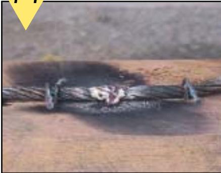
Braze the ends of the cables together. A steel coat hanger actually makes the best brazing rod for this step. The coat hanger will join the sections and still remain flexible enough to bend around the sheaves. Grind off excess material when finished brazing.
