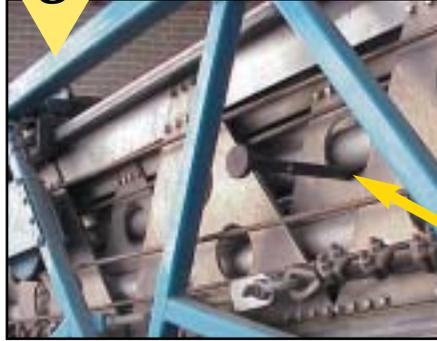
Place a large bar (see arrow) through the boom sections. This will keep the boom from retracting or extending as the cable is pulled.
