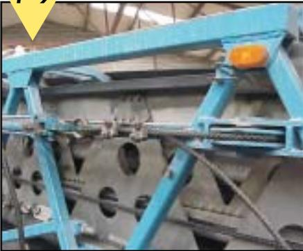
Move the tension cylinder toward the sheave and reform the loop with a thimble. Install the first clamp and pull enough tension to remove the clamp from the tension track.
