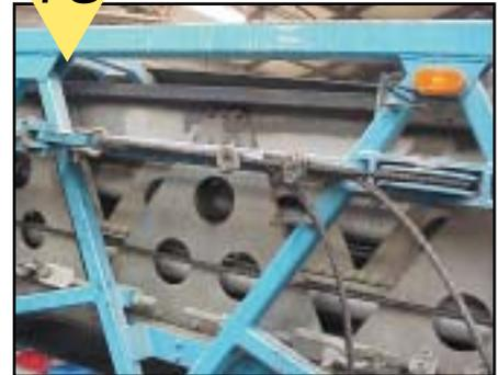
This photo shows the cable clamped to the tension track. This allows you to move the cylinder close to the sheave, so you won't run out of track before tensioning is completed.
