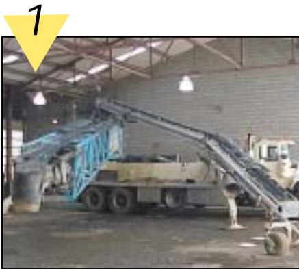
1 Position the machine and outriggers so that the feeder can be placed out of the way and the boom will be about 90° to the truck.
