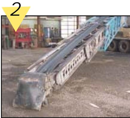
2 Extend the boom until the mid sections are extended a few feet to gain working room around the telescope drive assembly. Fully retract the tip section and lower the tip to the ground. Turn off the truck engine and put the keys in your pocket.
