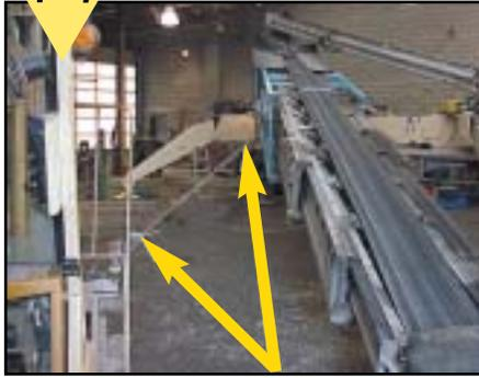
Three people are needed to pull the cable: one to feed the cable, one to operate the forklift and one to operate the Telebelt.
